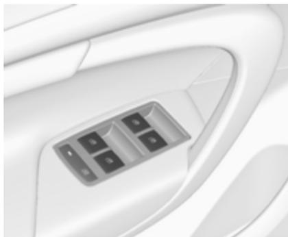
Pressionar o interruptor
