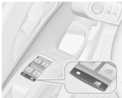
Pressionar o interruptor
